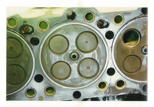
Exhaust valve on left wiped clean with no carbon build-up on stem.
