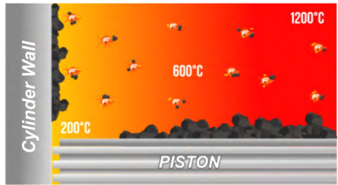
This graph shows the typical temperatures in the combustion chamber of an engine, looks like ferox molecules disperse and modify the activation temperature of the fuel and existing carbon deposits to achieve a complete and effective combustion.
